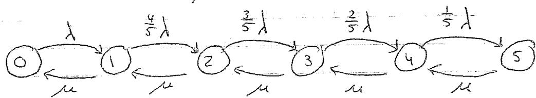
$$\begin{aligned} \lambda p_0 &= \mu p_1 \\ [\mu + \lambda(1 - \frac{i}{5})] p_i &= \lambda(1 - \frac{i-1}{5}) p_{i-1} + \mu p_{i+1}, \quad i=1,2,3,4 \\ \frac{1}{5} \lambda p_4 &= \mu p_5 \end{aligned}$$
