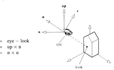
${\tt gluLookAt}$  normalizes n,u,v to unit length and uses the normalized vectors to build up the viewing matrix:
