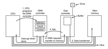
3b The disk controller for DMA has an internal buffer. Why is this buffer needed?
