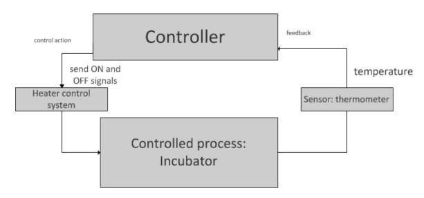
The control action is Send ON and OFF signals. For this control action we build a table for unsafe control actions.
