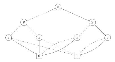
Eliminate nodes of which the 0- and 1-transition lead to the same node (C2, two times).
