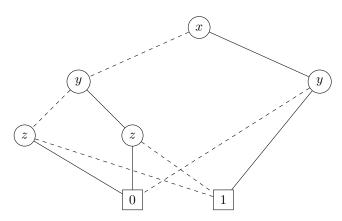
Collapse nodes that have identical 0-and 1-transitions.
