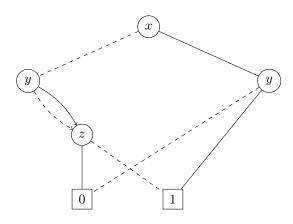
Eliminate nodes of which the 0- and 1-transition lead to the same node (C2).
