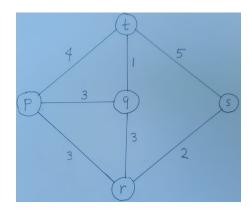
Note that three channels have the same weight. To avoid deadlock, we define an ordering on these channels: pq < pr < qr.
