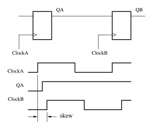
In the absence of clock skew, flip-flop B records a 0 at the first clock edge. However, if Clock B is delayed as shown, the flip-flop records a 1.
