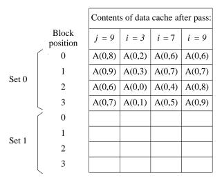
In all 3 cases, all elements are overwritten before they are used in the second loop. This suggests that the LRU algorithm may not lead to good performance if used with arrays that do not fit into the cache. The performance can be improved by introducing some randomness in the replacement algorithm.
