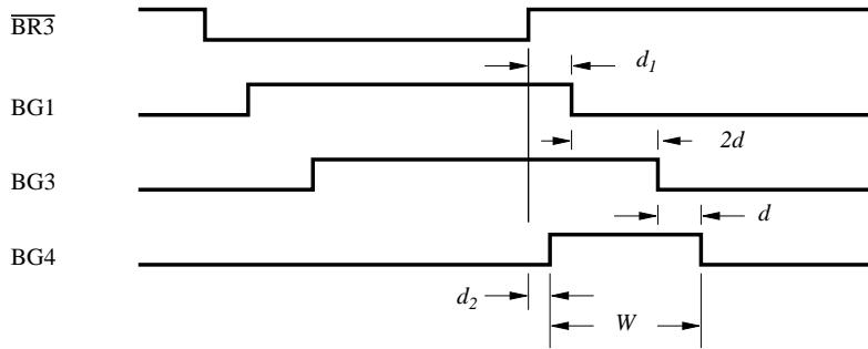
Assuming device 3 asserts BG4 shortly after it drops the bus request (delay  $d_2$ ), a spurious pulse of width  $W = d_1 + 3d - d_2$  will appear on BG4.
