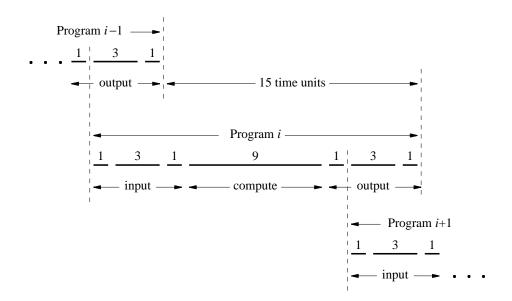
Time between successive program completions in the overlapped case is 15 time units, while in the non-overlapped case it is 19 time units.
