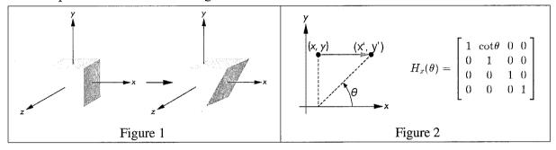
a) Implement a Java method that manipulates OpenGL's Current Transformation Matrix by way of the shearing matrix  $H_x(\theta)$ :
