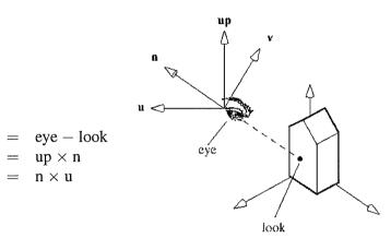
glulookAt first normalizes n, u, v to unit length and then uses the normalized vectors to build up the viewing matrix:
